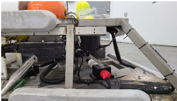
Figure 8: Platform with hydrophone guard installed
