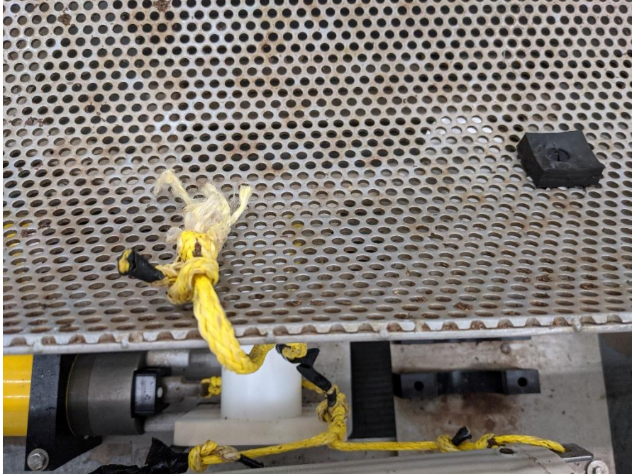
Figure 2. The chafed knot on one side of the spool cover.
