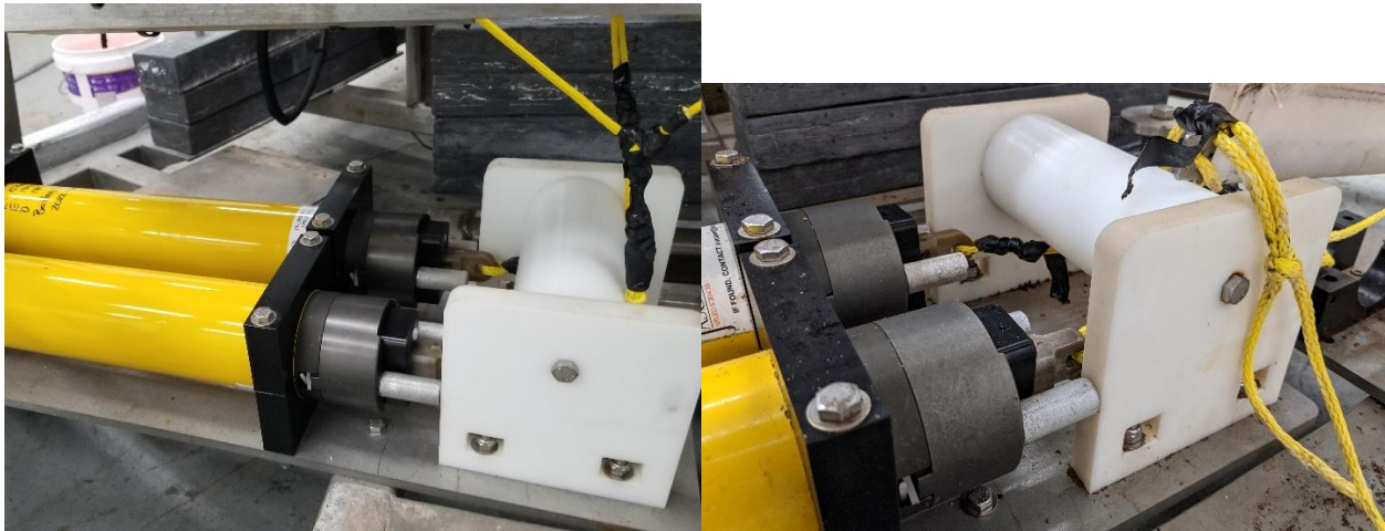
Figure 1. Release mechanism as rigged prior to deployment and post recovery.
