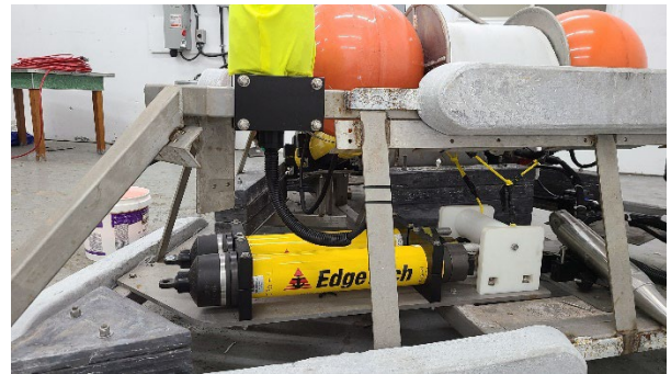
Figure 9: close-up of hydrophone guard (yellow plastic)
