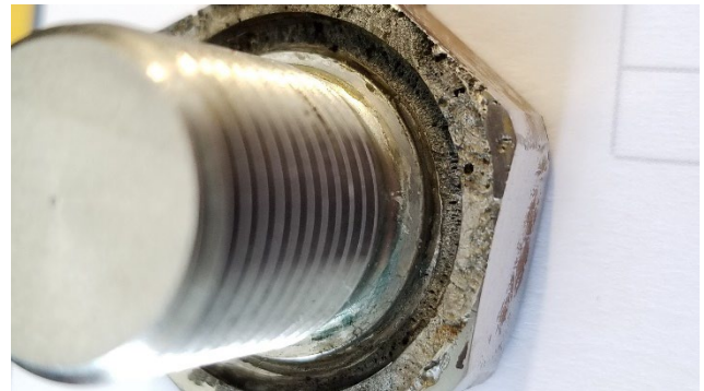
Figure 16: Corroded MUX plug, threads
