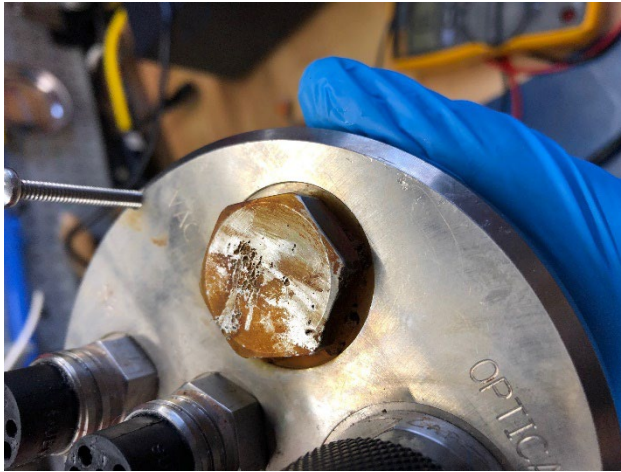
Figure 15: Corroded MUX Plug
