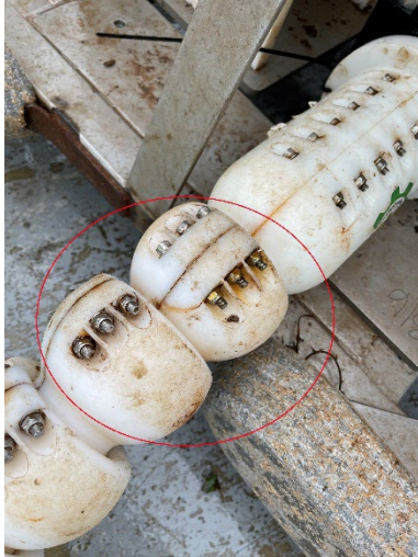
Figure 33: Crack in Bend Restrictor
